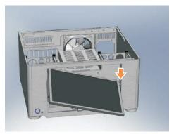
slide one side only of the TFT downwards as shown, until you see the roller bearing come free from the runner.
