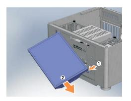
carefully (DO NOT FORCE) pull the right side slightly, so the bearing totally comes clear of the chassis (1), and then slide the whole TFT housing to the right, freeing the roller bearing on the opposite side.
