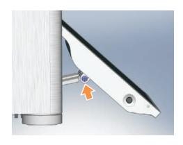
firstly, disconnect the TFT cable from the hub PCB on top of the motor housing and cut the cable tie that secures it to the TFT/motor arm. locate the screw as show on the left and remove.
