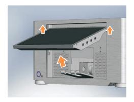
swing TFT housing away from the motor arm and roll upwards toward the top of the case until it almost touches.
