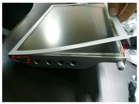
4. Remove front aluminum bezel as like picture. And front aluminum bezel might be bended, remove it very carefully.
