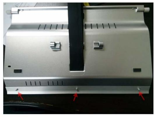
2. Remove 3 x round head screws on bottom.
