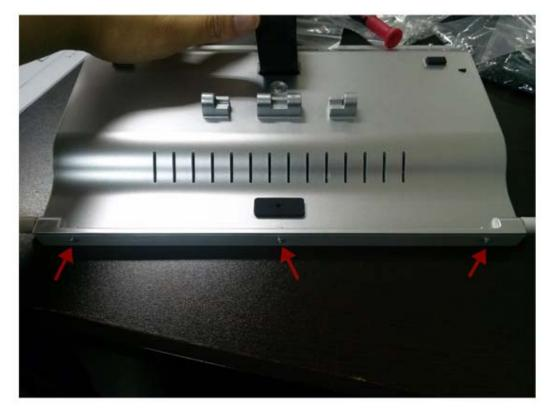
1. Remove 3 x flat head screws on top.
