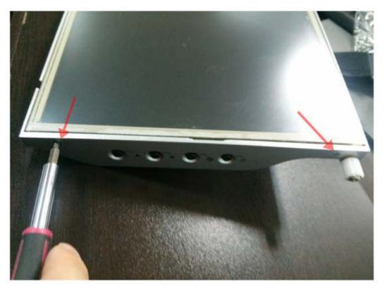
3. Remove 4 x round head screws on each side.
