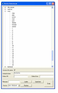
The checkbox "Device DB active" allows to switch the IR Database on or off.
