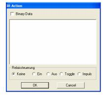
The Relay Control allows controlling the integrated relay via IR Commands. The options can be used to switch the relay On (On), Off (Off), to toggle it (Toggle) and to pulse it (Pulse).
