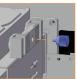
\*A fifth drive can be installed to the S16V, using the HM100 hard drive mount (optional).
