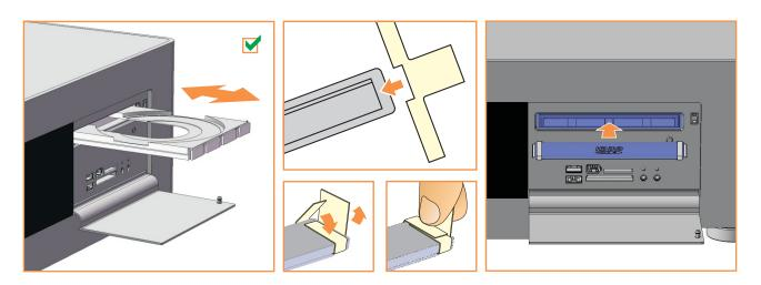
Check that the drive has been aligned correctly and that the tray can eject and close freely. Peel the back off the adhesive foam strip on the rear of the aluminium bezel. Fold a cardboard spacer around each end of the bezel, holding your thumb against the flaps as shown. With the tray closed, position inside the drive opening and press firmly against the front of the tray to ensure good adhesion. Eject the tray to remove the spacers (a gentle tug may be required).
