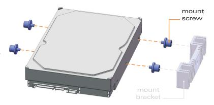
To install drives 1,2 and 3, begin by removing the two thumb screws...
