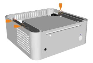
The HDD/ODD cage can now be secured to the chassis using 7 screws in total, 4 at the bottom and 3 on top as shown in the diagram. Note that 2 of the screw underneath fix to the 2.5" hard drive (shown in red), so ensure the correct screws are used.
