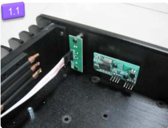
1.1 Install IR receiver by accessories' screws, showed on page 2
