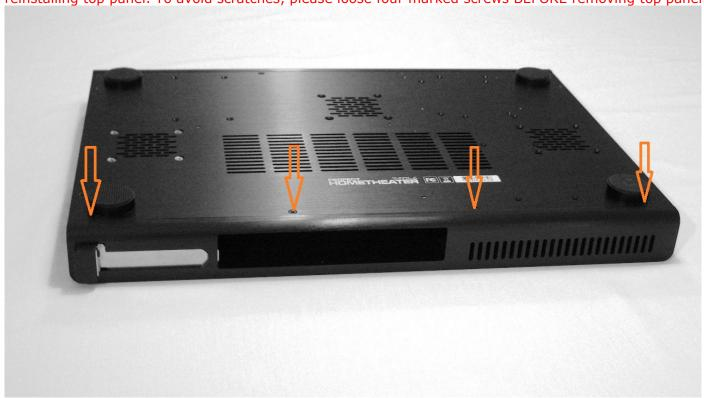
Now, when back panel is loose, you can remove and reinstall top panel without making any scratches. After your assembly is finished, please tighten all four screws gently.
